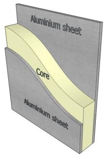
Some manufacturers have produced sandwich panels that have been subject to independent fire testing and approval. This may not mean they are 'non-combustible' but does demonstrate an improved fire performance.
